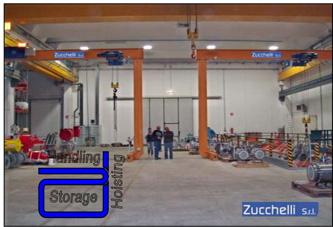
Gru a Portale Zoppo con Testata a Terra a ruote gommate Semi-Portal bridge crane with Rubbered Head
